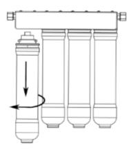
d. Remove the cartridges/membrane from their original packaging. Each cartridge and/or membrane must be placed in the corresponding position maintaining the correct order. To do so, you must insert each cartridge in its cap and turn it anti-clockwise. This process must be carried out for each of the cartridges that you want to replace.
